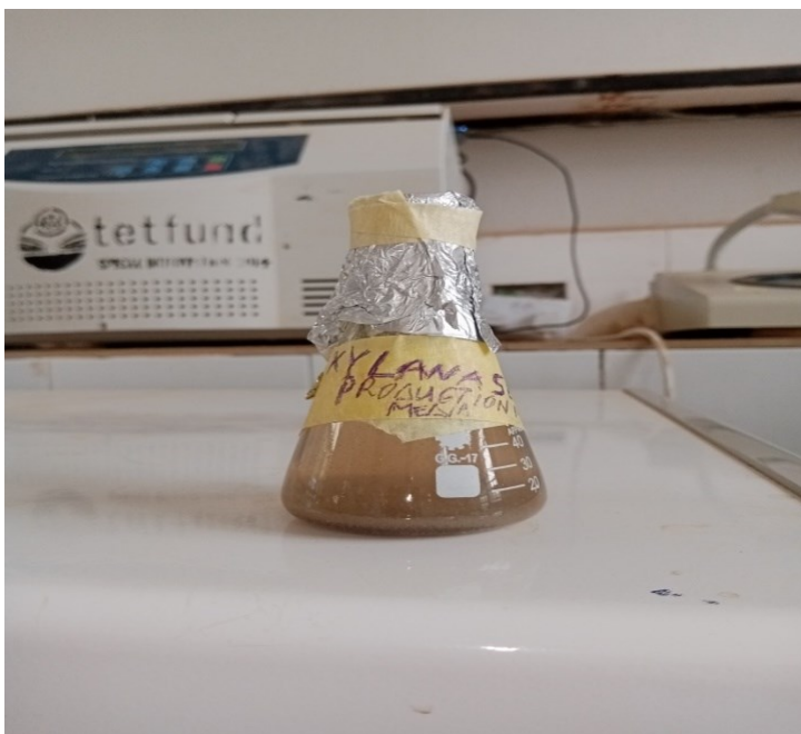
Fig 3: Submerged fermentation culture for enzyme production.
